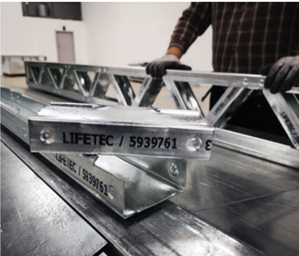
LIFETEC CONSTRUCTION GROUP LifeTec Construction Group takes rolls of steel and mills them into a package of steel joists and studs by using a 3D printing concept customized on a project-by-project basis.
